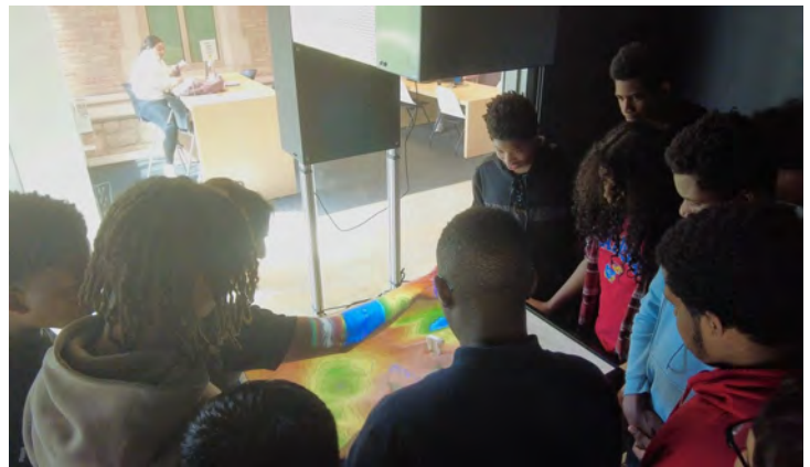
A UMKC sandbox projects colored contour lines as students create mountains and valleys.
